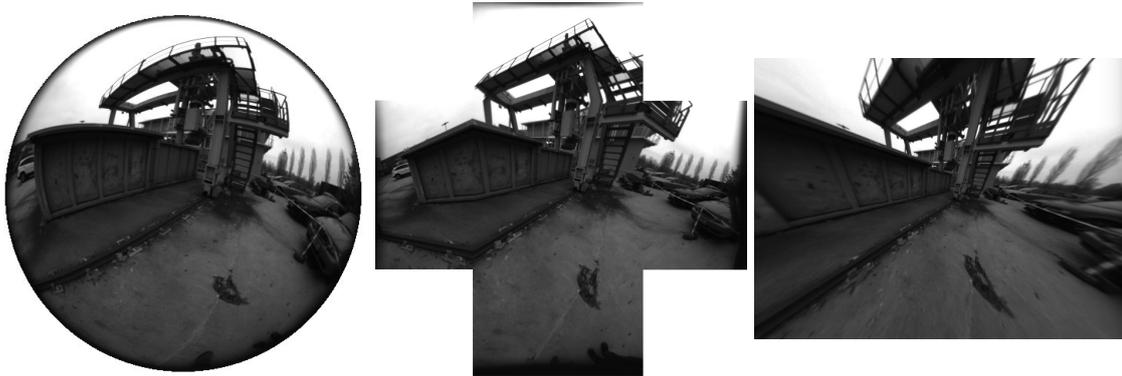
Figure 7.2: **Camera Models.** The same image, warped to fit the three projection models considered in this paper. While the Unified model and the piecewise rectified model can cover the full  $185^\circ$  field-of-view, the pinhole model shows significant distortion – when cropping the image to a field-of view of only  $120^\circ$  horizontally, as done for this figure.
