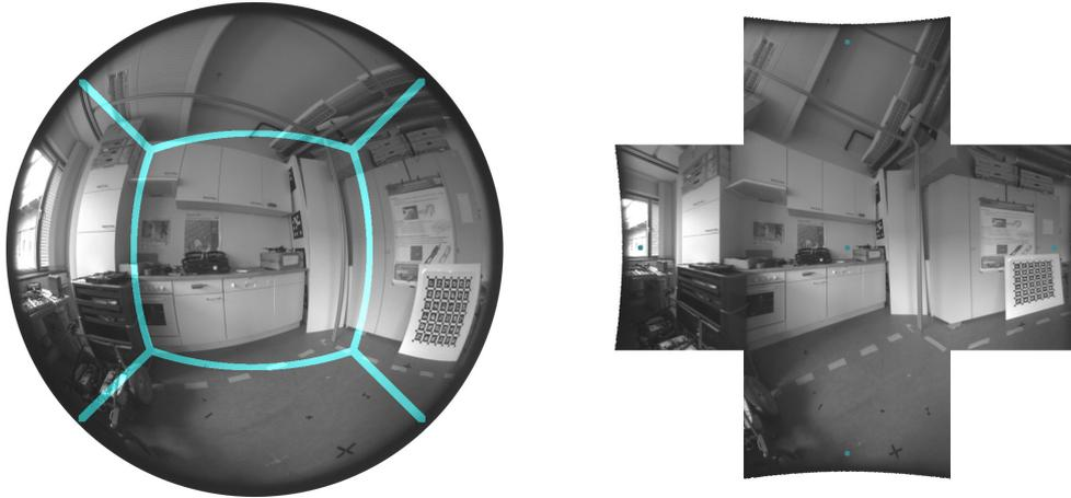
Figure 7.7: **Piecewise rectification.** Example of fisheye camera rectification. The borders are still distorted, as it is clearly visible on the checker-board, which leads to interpolation artifacts or blur.
