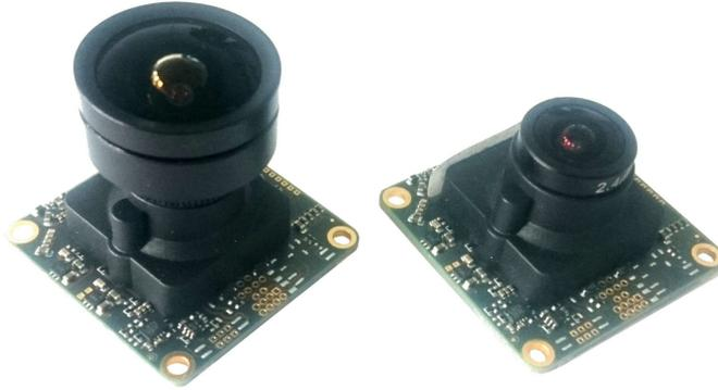
Figure 9.2: **Cameras used to capture the dataset.** Left: narrow lens ( $98^\circ \times 79^\circ$  non-rectified field of view), right: wide lens ( $148^\circ \times 122^\circ$  non-rectified field of view).
