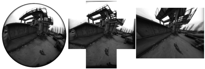
Fig. 2. Camera Models : The same image, warped to fit the three projection models considered in this paper. While the Unified model and the piecewise rectified model can cover the full 185^\circ field-of-view, the pinhole model shows significant distortion – when cropping the image to a field-of view of only 120^\circ TODO diagonal or in x-direction?, as done for this figure.
