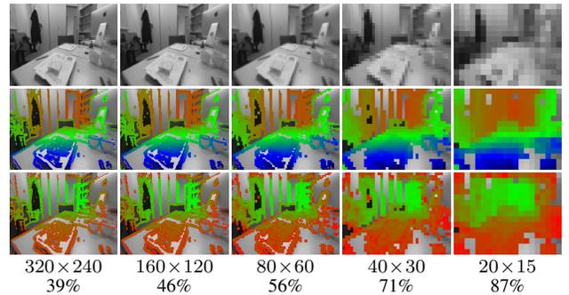
Figure 5: Image Pyramid. Top: intensity image  $I_l$ , middle: color-coded inverse depth  $D_l$ , bottom: inverse depth variance  $V_l$ . The given percentage corresponds to the density, i.e., the percentage of pixels that have a depth value. The described down-sampling strategy causes the depth maps to become significantly denser on higher pyramid levels.
