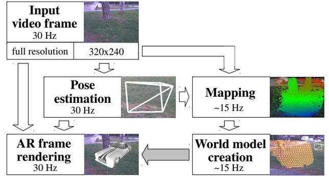
Figure 7: AR Processing Pipeline: Camera images are retrieved and displayed directly at full resolution. Simultaneously, a downsampled ( $320 \times 240$ ) version is computed and processed in the VO pipeline to allow real-time tracking and mapping. The estimated pose of that frame, as well as the generated world model are then used to render virtual objects into the scene. The world model is updated asynchronously at a lower frequency. All components run in parallel.
