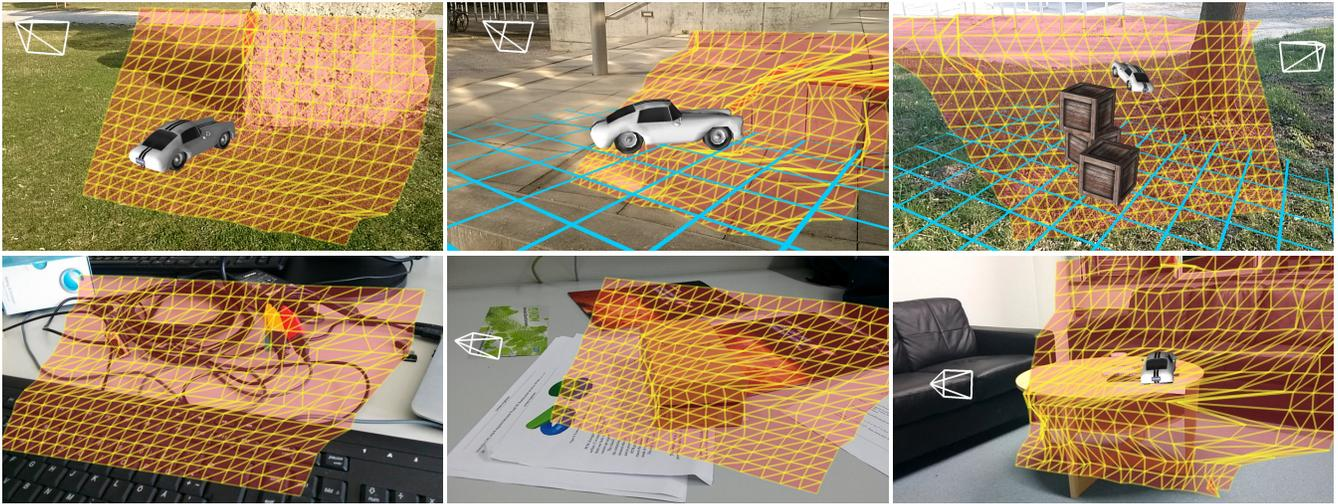
Figure 9: Qualitative evaluation of the system in different, challenging scenes. The collision mesh is fixed and shown from a different perspective, together with its original viewport, augmented objects and the ground plane. The screenshots are taken by the smartphone during live operation.
